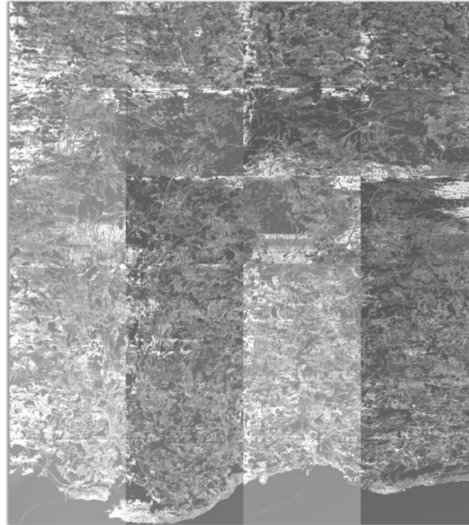
FIGURE 6. SEM COMPOSITE PICTURE OF THE SECTION OF THE FABRIC IMPREGNATED WITH THE COAGULATED PUD.
